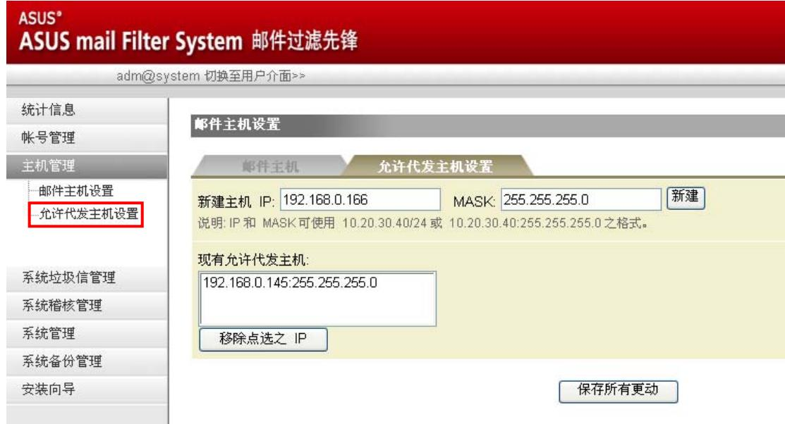
The screenshot shows the 'ASUS mail Filter System 邮件过滤先锋' interface. The left sidebar has a 'Host Management' section with 'Allow Relaying Hosts' selected. The main content area is titled 'Allow Relaying Hosts' and contains fields for 'New Host IP' (192.168.0.166) and 'MASK' (255.255.255.0), a 'Create' button, and a note about IP and MASK formats. Below this is a table showing existing hosts (192.168.0.145:255.255.255.0) with a 'Delete' button. A 'Save All Changes' button is at the bottom.
